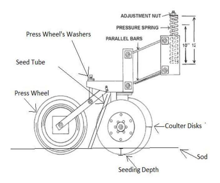
Once you have calibrated your seeding rate, it is time to adjust the drill to the appropriate seed depth. Plant a few feet and check the depth of the trench with a ruler.
