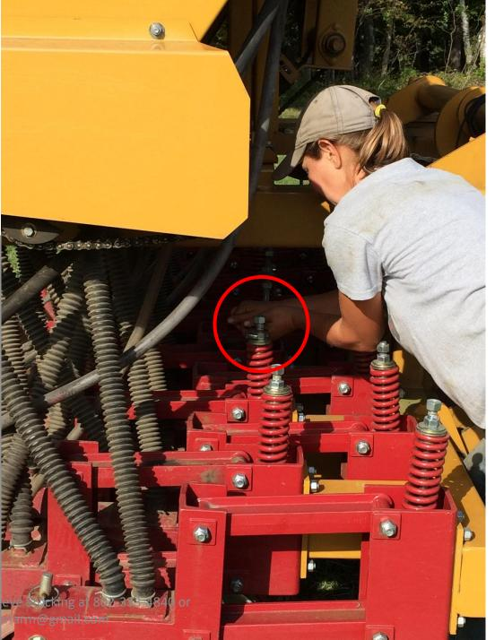
The springs should be compressed between 10-12 inches in length; do not tighten the nuts to compress the spring to less than 10 inches in length in order to avoid excessive tension that will damage the openers.
