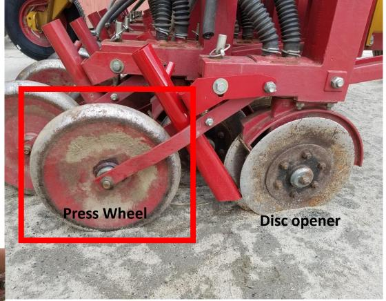
Raise the press wheels by moving washers from the bottom of the pin to the top; to lower them, move washers from top to bottom. Repeat for all press wheels.
